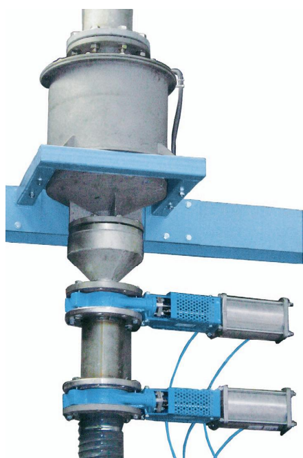
Heavy medium hydrocyclone
